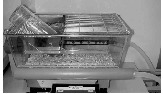
Fig 1 The specially designed type III cage for use in the air speed studies. Ten holes were made in each side of the cage. In front of the holes, on the outside of the cage, a PVC tube was placed with an opening into the holes. One end of the tube was closed, and the other end was connected to a silicone tube. The silicone tubes were connected to a ventilator giving 50 air changes per hour. With all holes opened, the air speed at animal level was less than 0.2 m/s, and with every second hole opened, the air speed at animal level was 0.5 m/s
