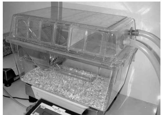
Fig 2 The type III cage with the special designed filter top for use in the air change studies. The filter was replaced with plastic parts, and a special chamber was designed in one half of the filter top. The front of the chamber was equipped with filter and the back of the chamber with two connections for silicone tubes. The silicone tubes were connected to a ventilator giving 50, 80 or 120 air changes per hour
